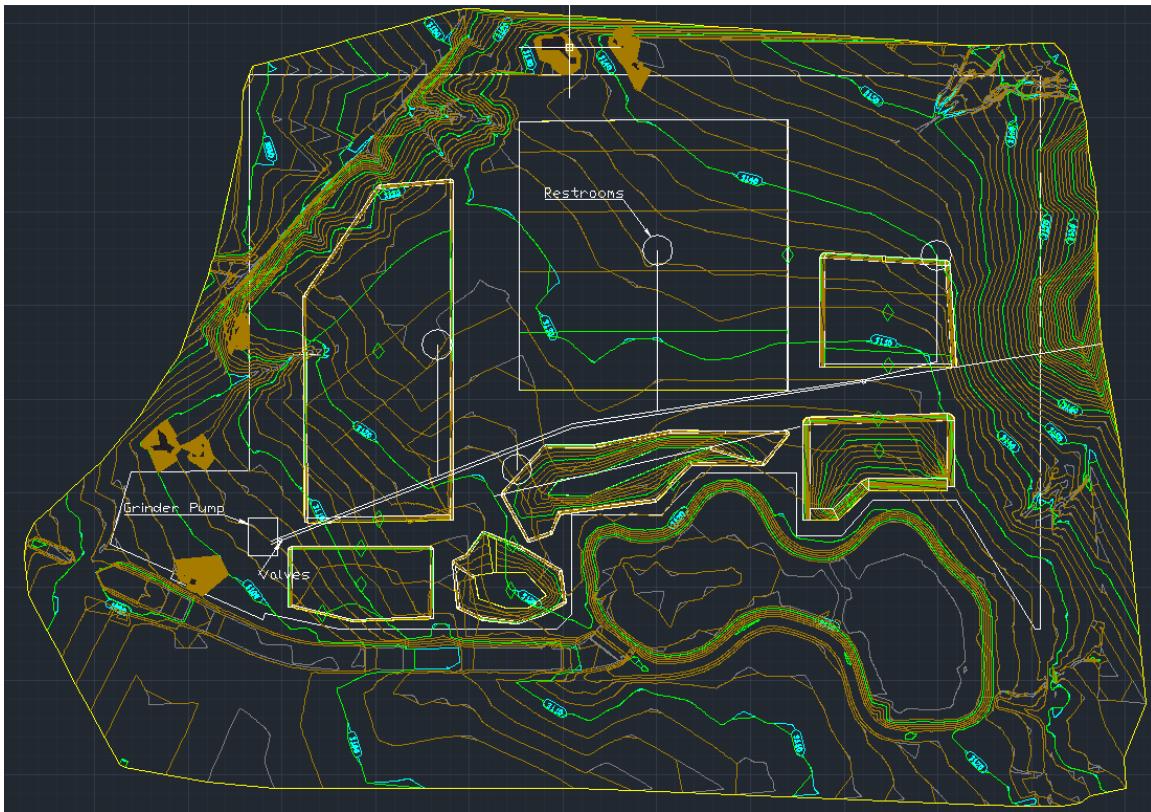
Figure 4.2- finished wastewater plan view
